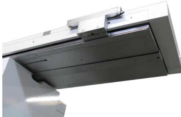
Illustration 6.2: Electromechanical safety switch at a Block-examination unit
