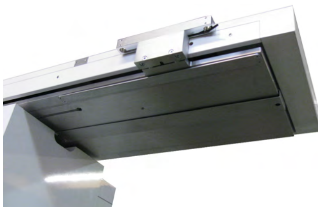
Illustration 8: Electromechanical safety switch
